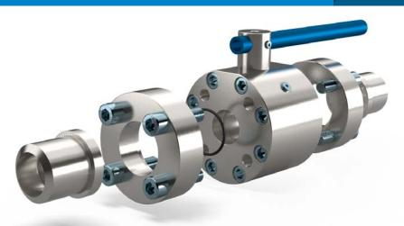
**MHA** ZENTGRAF offers flange ball valves including welding ends with pipe Schedule XXS, 160, 80 or special pipe sizes upon request. The flanges are manufactured by **MHA** ZENTGRAF with full material traceability through 3.1. mill certificates.
